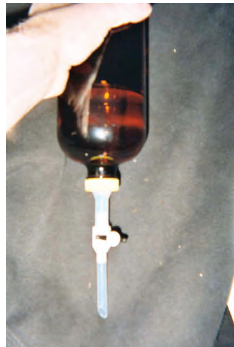
Figure 2 Photograph of bottle cap attachment enabling phase separations to be conducted directly in bottles.
