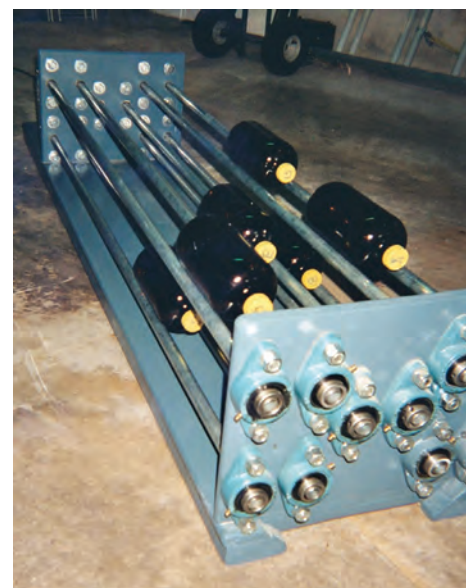
Figure 1 Photograph of prototype BLLE bottle rotation device.
